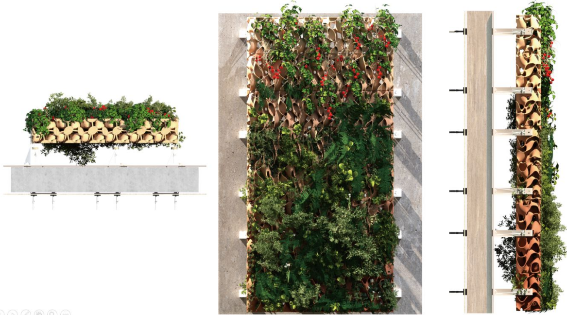
Figure 10. Structure of secondary façade applied to a retrofitted building (render)
