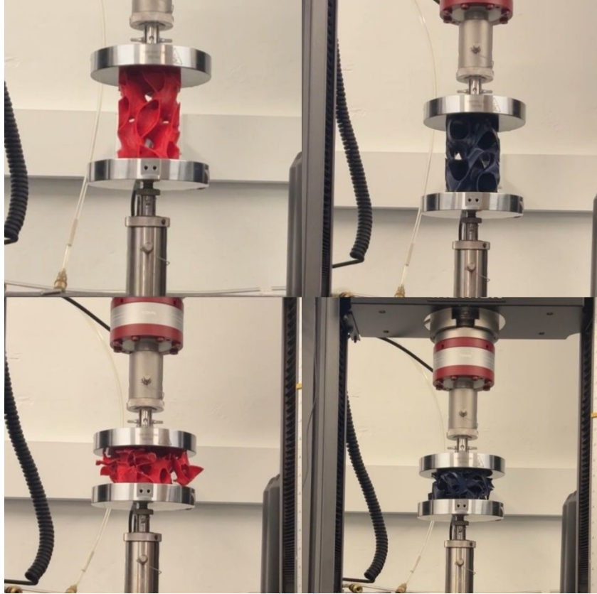
Figure 13. Compression test – before and after loading.
