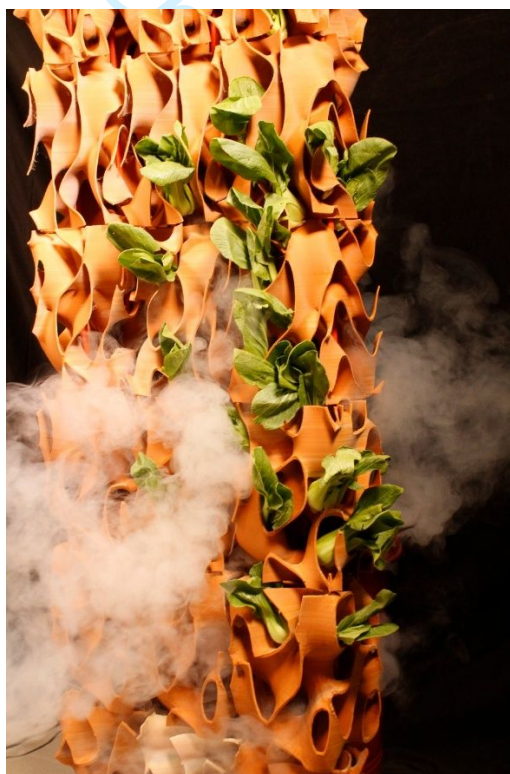
Figure 9. A real-life photo demonstrating how nutrient mist irrigates the clay façade.
